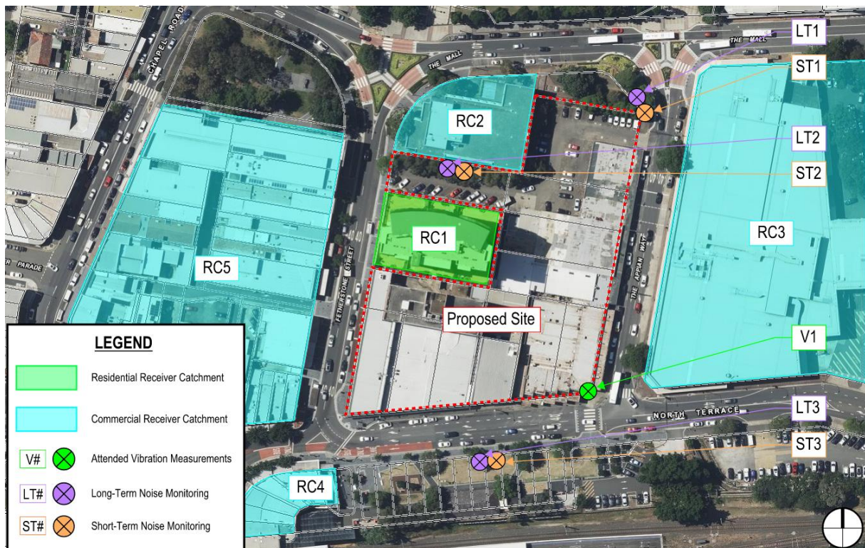
Figure 3: Acoustic site plan identifying the surrounding noise-sensitive receivers and noise monitoring locations
